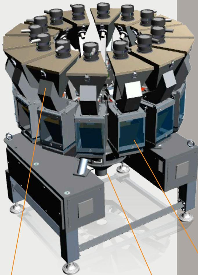
**1** Up to 14 individual weighing channels gravimetrically release a controlled amount of material from the material hopper into the weighing station.
