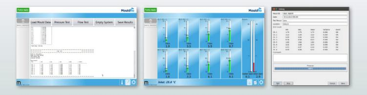
By using the Test-rig you are able to generate a full report with printed documentation validating all of the flow and pressure characteristics within the mould.
